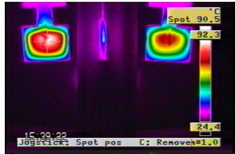
Thermal Imaging of PLED ( 0.1\text{cm}^2 )
